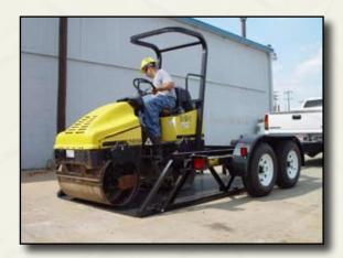
The adjustable hitch on the trailer makes it possible for the operator to move the coupler to accommodate any hitch height on the towing vehicle. This operation is as simple as removing two bolts, adjusting the coupler and replacing the bolts.
