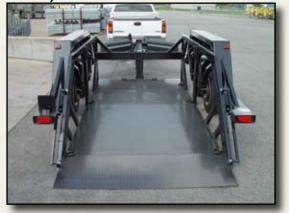
Featuring a welded heavy duty frame, powder coated paint finish and a heavy duty diamond treaded plate deck, this trailer is manufactured to give years of durable, reliable service.
