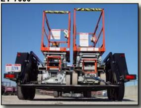
The wide deck on the ET 12,000 allows for more equipment to be loaded at one time. Larger equipment can also be accommodated with this trailer.
