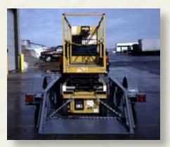
Escalate Trailers from Bil-Jax save loading and unloading equipment time since the deck hydraulically lowers to ground level. Equipment can be loaded by one person, even in inclement weather.
